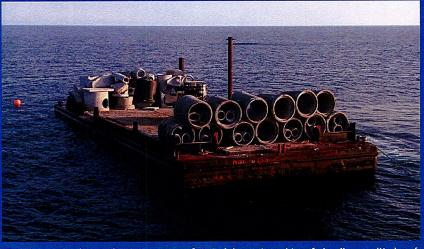
Barges carrying large, clean concrete reef materials are towed to a federally permitted reef construction sites offshore where material is deposited on the seabed, forming an artificial
